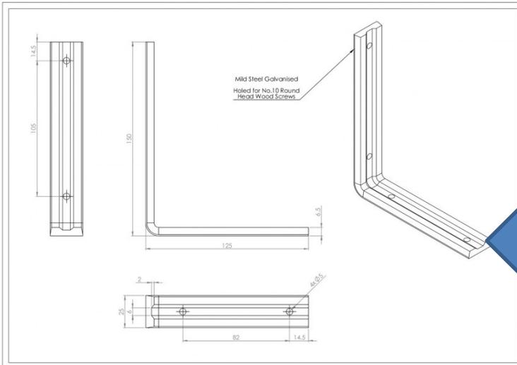
Only one screw per bracket is used to fix the Window Box to the bracket.
